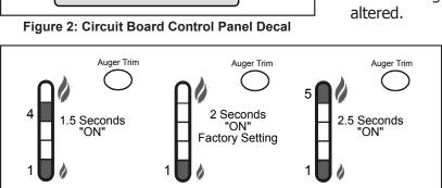
Figure 3: Auger trim and heat level indicator.
